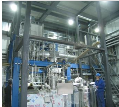
High-temperature fluoride salt experimental loop
